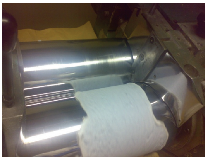
Fig. 1: The production of abaca fibre reinforced HIPS composites using a rolling machine
